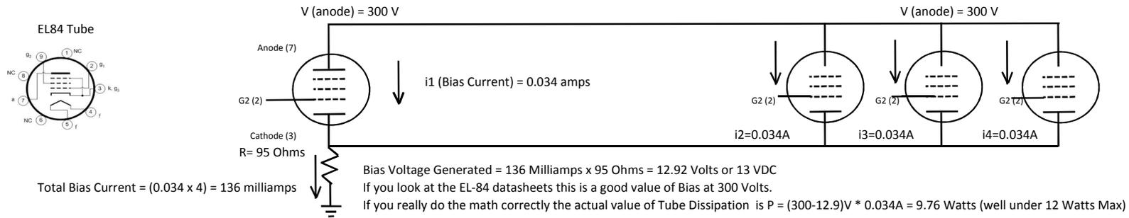
In the above example, I have 287.1 Volts on the Anode (Plate) of the ST-35 Output Tubes and all 4 Cathodes tied together through a 95 Ohm Bias Resistor.
