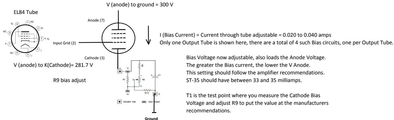
The reason why we don't see adjustable Cathode Bias is the potential damage that setting the controls can do to the amp. The same can be said about Fixed Bias adjust, damage is also possible there as well. So knowing how to properly adjust Bias and knowing when you need to buy matched tubes is key.
