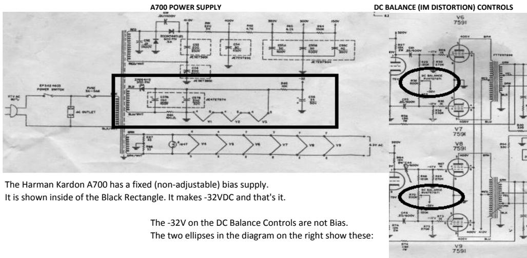
The Controls in the Ellipses are DC Balance, not Bias. They are like a very fine DC offset. By changing the DC voltage by 1-3% you can dramatically attenuate I.M. Distortion.
