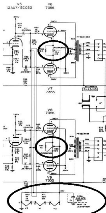
The Controls in the Ellipse are DC Balance or IM Distortion settings, not Bias.
