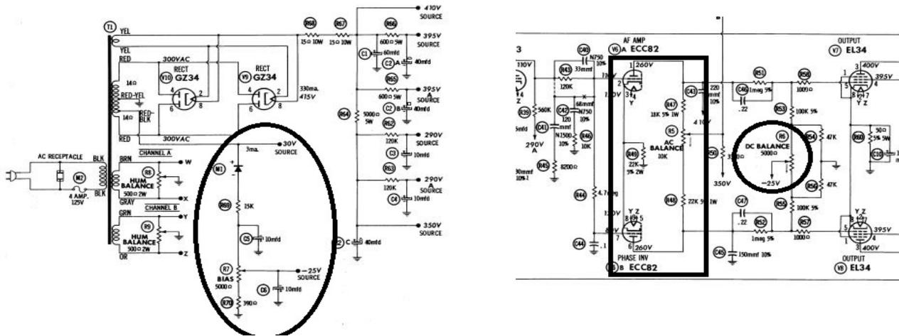
In the above we have the famous Fisher SA300. You can see from the Power Supply that there is a wire labeled 14 Ω Red-Blk. That is a Bias Tap, same as the ST-70. Then it produces 30V at the input to the Rectifier Diode. Then a series of resistors and a Bias Control R7 provide a adjustable bias supply of -25V according to the setting on the schematic.
